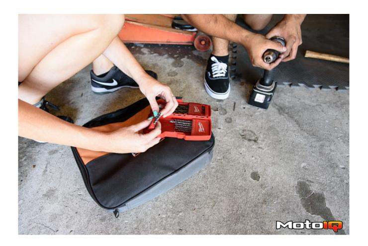
There really isn't any science behind choosing the right drill bit for the job since our mounting screws are pretty small in diameter. We chose our best drill bit available that was smaller than the mounting screws, yet not broken and not too dull.
