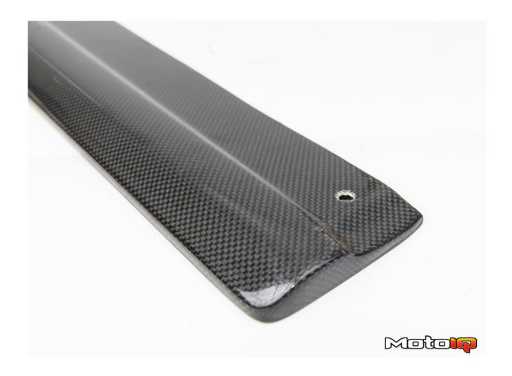
The edges are finished very nicely. This rear facing end lines up very nicely against the pinch weld and rear of the rocker panel. The rear of the rocker panel has a small bracket that hangs, which is a good reference point to utilize for mounting.
