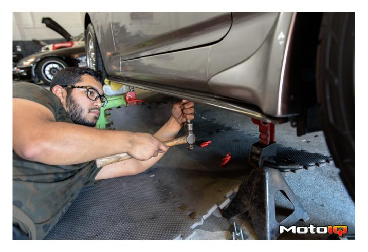
Now that the diffuser is held in place with the double-sided tape, it makes it very easy to finish the installation by drilling the screws into place. Each side uses five mounting screws. Here, Vince uses a center punch to create a guide for the pilot hole.
