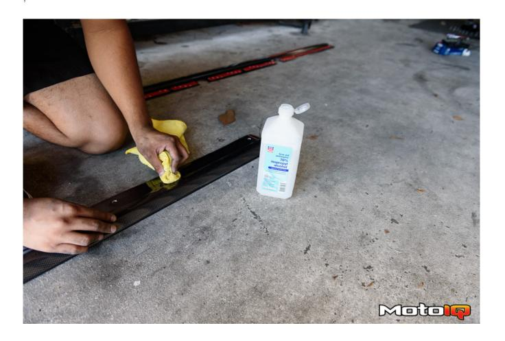
We highly recommend using double-sided 3M tape for the install. This will make your life much easier when drilling. In order to get a good adhesion, wipe the area with alcohol first.
