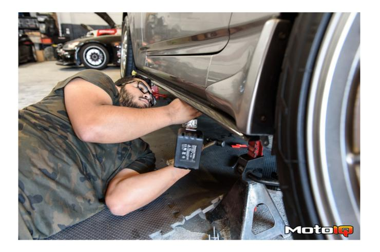
After drilling the pilot holes, Vince drills the five mounting screws to complete the installation of the first side.
