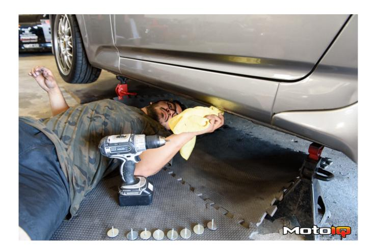
Don't forget to also wipe the underbody where the tape will be, otherwise, the tape will not adhere to the dirty surface. You won't be able to clean it perfectly, but a little bit can go a long way in this case.
