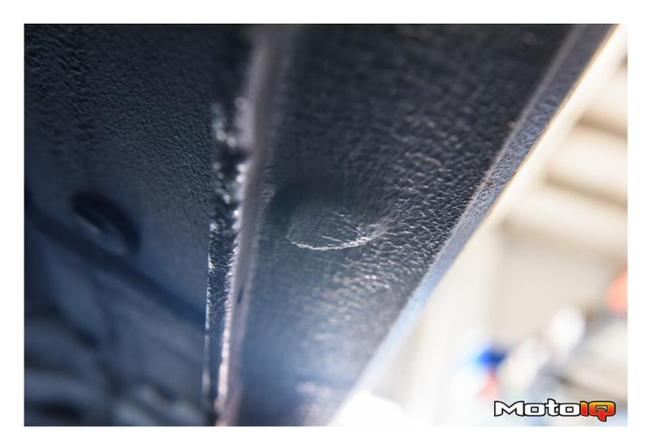
Each side of the S2000 has three small protrusions located just in front of the pinch weld along the under side of the rocker panel, as pictured here. They typically make fitment poor from other side diffusers, as they cause small gaps between the surface level changes.
