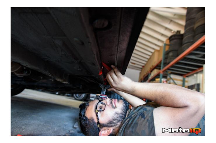
Remember the pro tip about not ripping off the whole backside of the 3M tape? Here, you can see that the backing of the tape casually folds downward while mounting. You can begin pulling the strips of backing once you are satisfied with the mounting location. They pull easily, and then firmly press the diffuser to fully set the adhesion of the tape.
