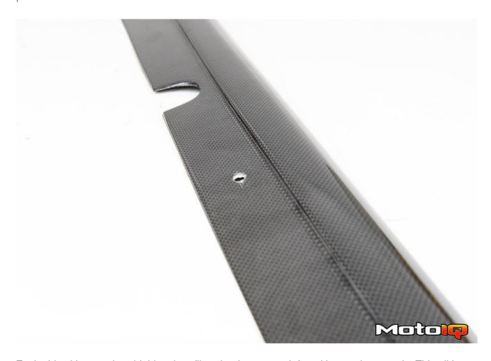
Each side skirt uses hand-laid carbon fiber that is vacuum-infused in a carbon matrix. This all happens at their facility in Long Beach, California.
