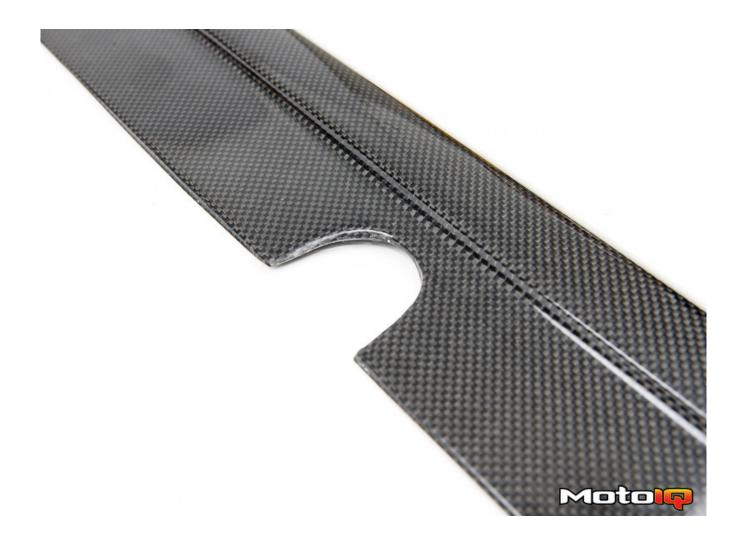
Not to worry, these diffusers cleanly accommodate space just large enough for the diameter of the round protrusions and actually help a lot for mounting perfectly, as we will mention shortly.
