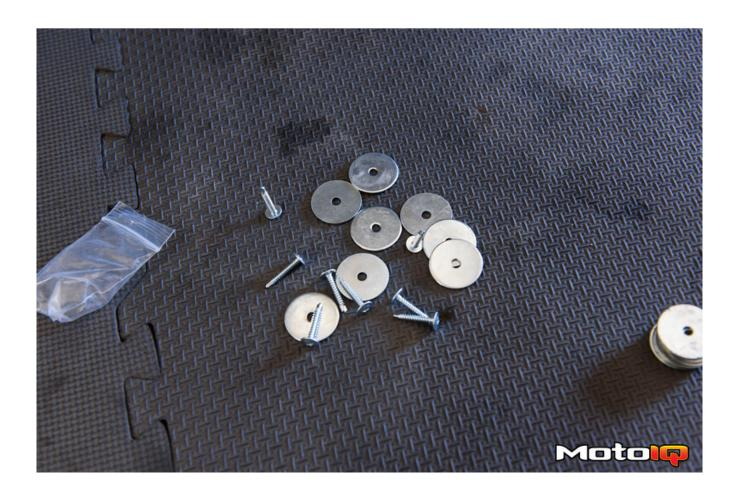
There is a good amount of margin of error with the provided hardware. The large fender washers combined with ample-sized drilled holes in the diffusers make it pretty easy to install.
